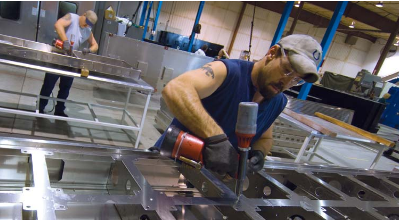
A Counterpart employee riveting a part in place.
